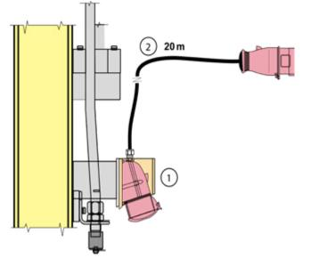
Picture 36: Protected booms socket and 20m cable to the magnet generator
