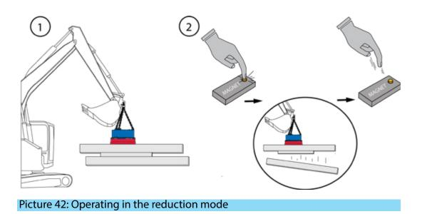
If button is released too soon (less than 0,5 sec.) the reduction mode won't activate and the magnet will fully demagnetize.
