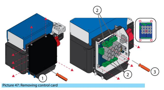
4. Apply the thermal paste provided with the card or quality termal paste to the bottom of the new card
