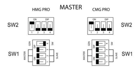
Picture 30: Single/MASTER card DIP switches
