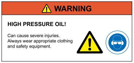
The hydraulic system is pressurized up to 420 bar.
