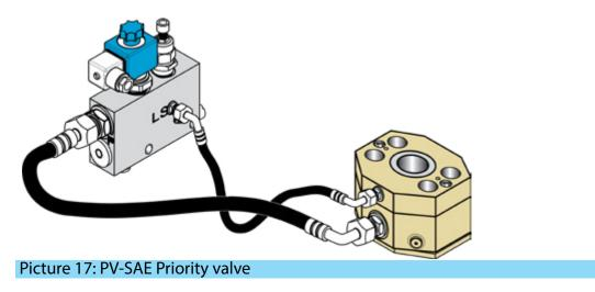
DYNASET PV- SAE priority valve enables the installations of the DYNASET products into any hydraulic system.
