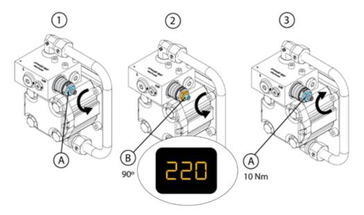
During the adjustment U.CUR will blink on the display. This is normal. Do not attach magnet on to the generator while measuring the voltage.
