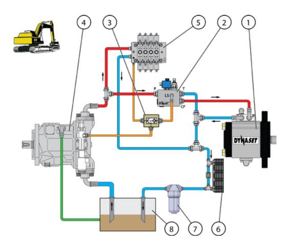
Picture 13: Connection figure for closed centre hydraulic system with load sensing variable displacement pump
