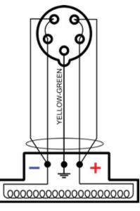
Picture 33: Wiring for the cable from the generator to the magnet
