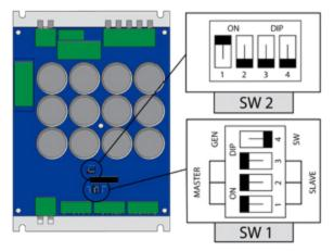
Picture 29: Location of the DIP switches on the control card
