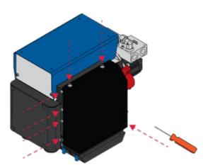
Kuva 49: Installation of control box cover.
