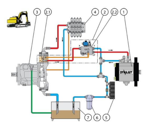
Picture 11: Connection figure for open centre hydraulic system with load sensing variable displacement pump
