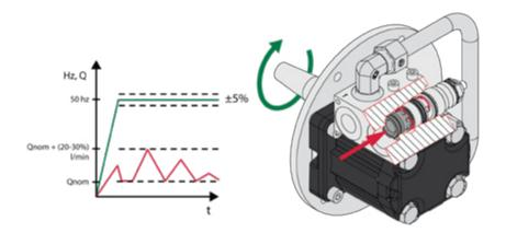
Picture 8: Automatic RPM-control
