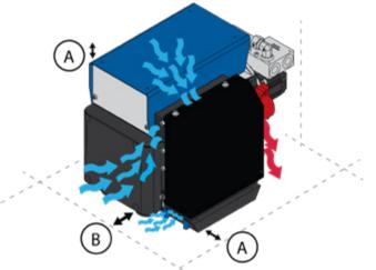
Picture 23: Placement of the HMG/CMG PRO hydraulic magnet generator.
