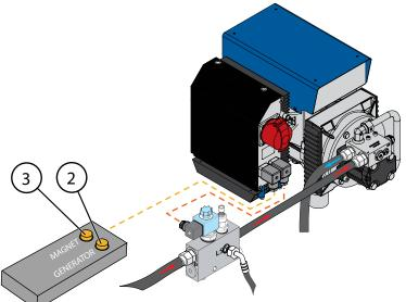
Picture 41: Operating the magnetization by controlling magnet generator's magnetizing voltage
